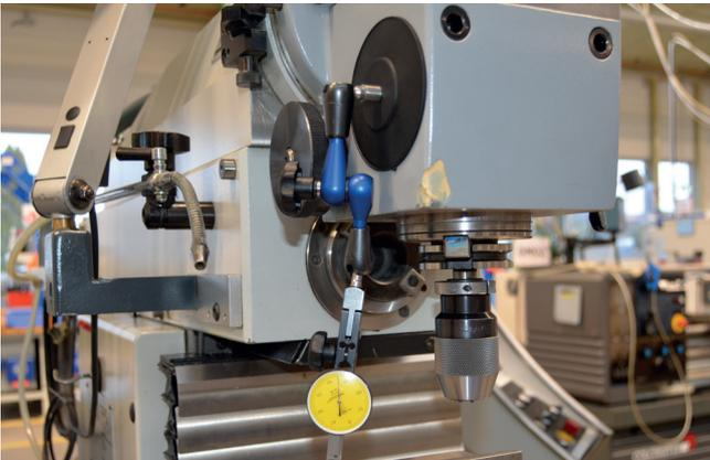
Fastening measuring devices to the machine housing
